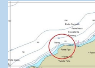
Figure 12 – Bathymetric conditions at Ana Chavez and Porto Neves (CMap) Draft at the quay needs to be at least: 10 meters
