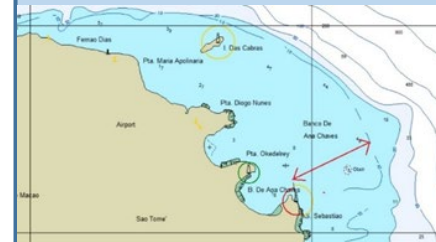
Figure 12 – Bathymetric conditions at Ana Chavez and Porto Neves (CMap) Draft at the quay needs to be at least: 10 meters
